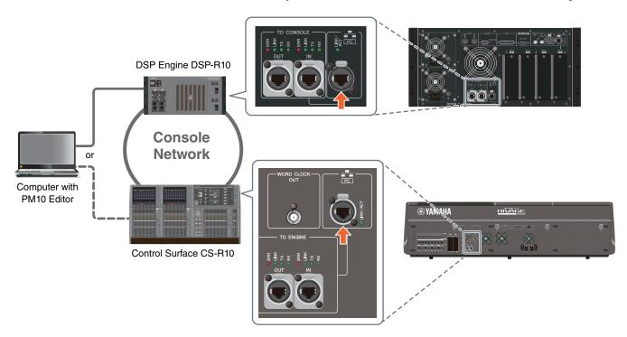
Connect the computer where PM10 Editor is installed to the DSP engine. To establish a connection with the DSP engine, connect the cable to the NETWORK terminal (PC) located next to the TO CONSOLE terminal. Never connect the cable to the NETWORK terminal above the HY card slots.
