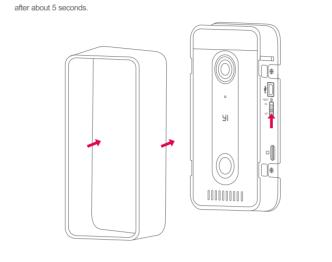
3. Charge for YI Video Doorbell 1) Plug the power cord with the power adpater into the side USB charging port; 2) When charging, the red indcator light up; When the electricity is full, red incator light off; 4) When you enter app, you can check the current electricity; Strongly suggestion:When first use the doorbell, charge for 4-5 hours until 100%.
