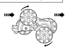
Press single joystick backward: spin with the side wheels revolve up and down
