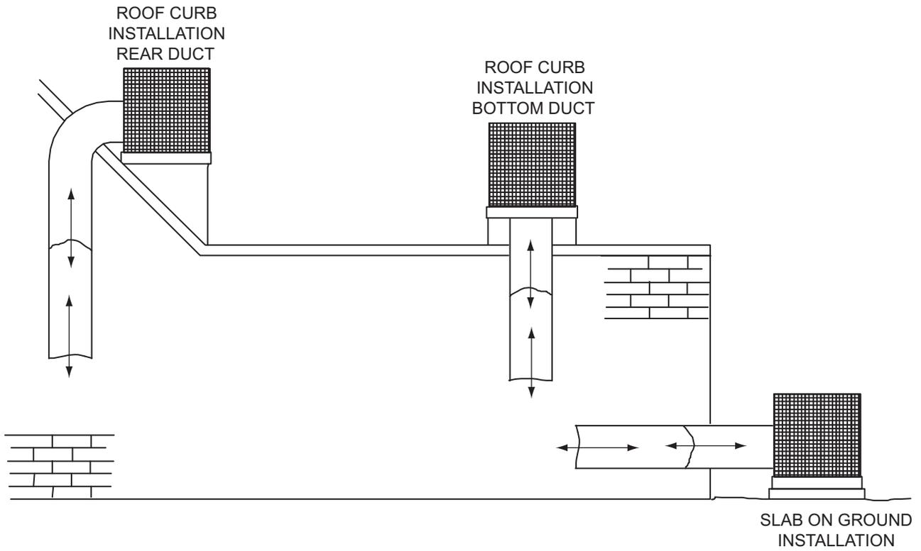
**Unit Typical Slab on Ground Installation**
