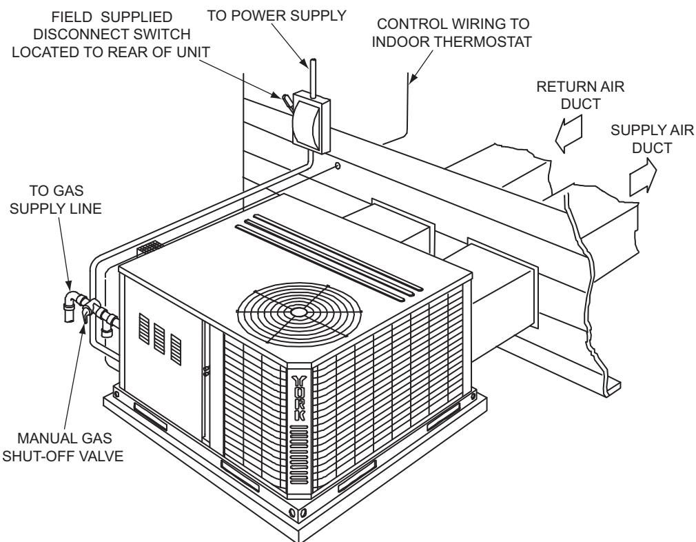
**Unit Typical Roof Curb Installation (Gas Model Shown)**
