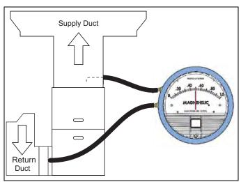
Set appropriate airflow per temperature rise for gas heating. Set appropriate airflow per Table 14 for cooling/heat pump heating operating based on outdoor unit size and external static pressure.
