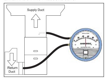
Set appropriate airflow per temperature rise for gas heating. Set appropriate airflow per "Blower Performance Table" for cooling/heat pump heating operating based on outdoor unit size.
