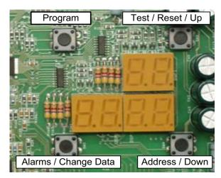
Figure 2: Simplicity<sup>®</sup> Controls Push Buttons
