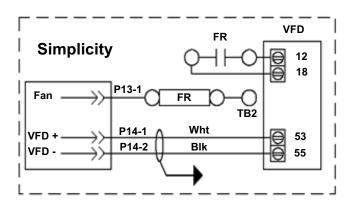
Figure 4: VFD Control Wiring
