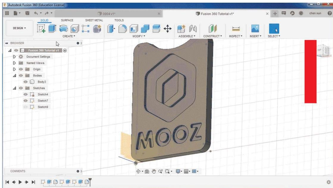
B. Use **Press Pull** tool to create the hanging hole feature.
