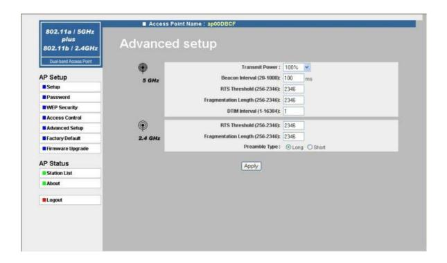
**Transmit Power:** Specifics the level of transmit power. Specify the value of the transmit power from the dropdown menu. You can set the transmit power for 100%, 50%, 25%,
