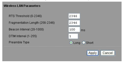
**RTS Threshold:** RTS Threshold is a mechanism implemented to prevent the "Hidden Node" problem. When the RTS is activated, the station and its Access Point will use a (RTS/CTS) mechanism for data transmission. The default setting is 2346.
