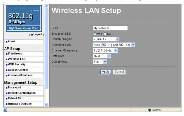
**SSID:** The SSID is a unique ID used by Access Points and Stations to identify a wireless LAN. Wireless clients associating to any Access Point must have the same ESSID. The default ESSID is "My Network". To change the SSID, type in the SSID you like to use. It is case sensitive and must not exceed 32 characters.
