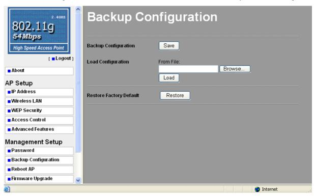
Note: the IP address settings will not be reset to factory default by this page. You should use the reset button of hardware or **Reboot AP** window if you want to reset everything including IP address into factory default.
