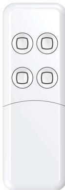
The Aeon Labs Minimote is a remote controller focused on enduser's ease of use. Although simplicity and user experience is the primary focus, the full range of Z-Wave remote controller capabilities are left intact for the advanced user. Network installation is vastly improved via the interface. The Minimote is upgradeable by the end-user such that the latest Z-Wave protocols are always available. An internal lithium battery allows for months of usage and is recharged via USB.
