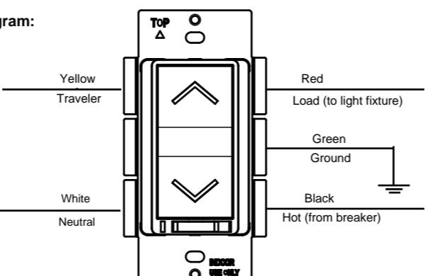
1. WARNING : To avoid fire, shock, or death. Turn off power at circuit breaker or fuse and test that power is off before wiring.
