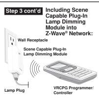
NOTE: Programmer/Controller must be in close proximity to Scene Capable Plug-In Lamp Dimming Module when including into network
