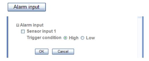
**Note:** You can set the alarm input function at alarm input page. (**Please go "Setting**  $\rightarrow$  **Advance**  $\rightarrow$  **Alarm input**  $\rightarrow$  **Setting"**). For more details, you can check Chapter 8.6.
