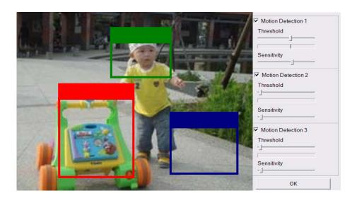
Note: You can set motion detection at motion detection page. (Please go "Setting  $\rightarrow$  Advance  $\rightarrow$  Motion detection  $\rightarrow$  Setting") For more details, you can check Chapter 8.7.
