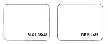
Press ENTER a third time to leave Tape Time Remaining display on TV screen. (REM indicates the time left on the video tape in the VCR—1:35 means one hour and thirty-five minutes are left on the video tape.)
