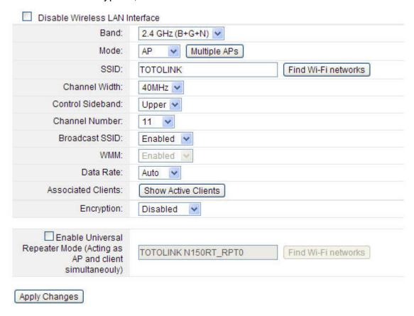
Click Multiple APs button, the multiple APs setup interface will appear. You can add other SSID for different needs. What's more, you can setup different encryption for different SSIDs in Security Settings section. We will introduce in **5.2.2 Security Settings**
