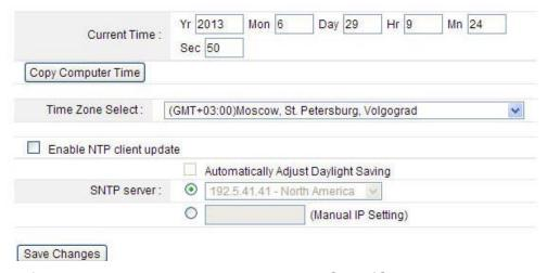
You can specify the device's time zone according to GMT (Greenwich Mean Time) or copy computer time as the current time only by clicking the **Copy Computer Time** button.
