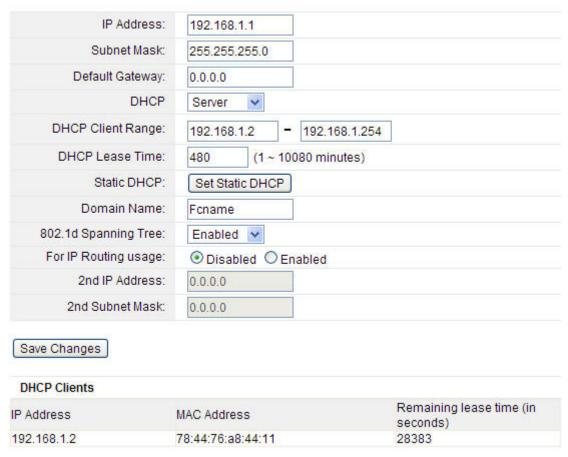
**IP Address:** This is the IP addresses to be represented by the LAN (including WLAN) interface that is connected to the internal network. This IP will be used for the routing of the internal network (it will be the Gateway IP for all the devices connected on the internal network).
