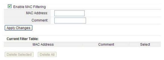
**Enable MAC Filtering:** you can check the box to enable MAC Filtering function.
