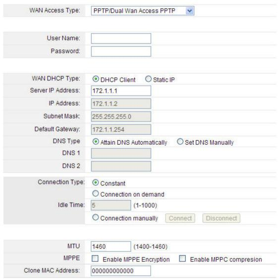
**WAN DHCP type:** it's available only for PPTP connection. If your ISP provides an extra type to connect to a local area network such as **DHCP Client/Static IP**, you should select the type and enter the right parameters provided by ISP to enable the secondary connection.
