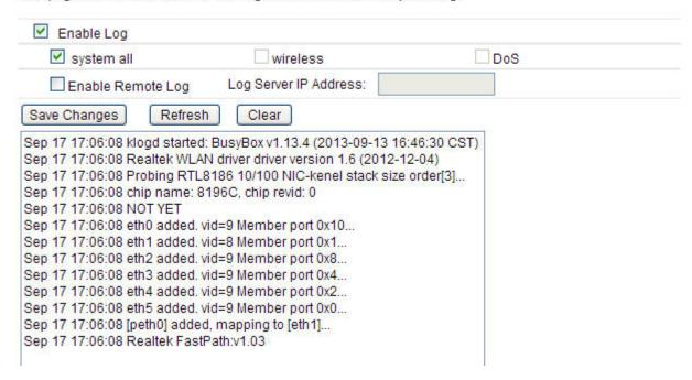
**Enable Log:** this option enables the registration routine of the system log messages. By default it is disabled. Below items including system all, wireless, Dos allows you to choose the log type.
