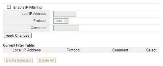
**Enable IP filtering:** you can select this checkbox to enable IP Filtering function.
