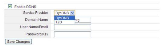
**Enable DDNS:** please select this checkbox to enable DDNS function.
