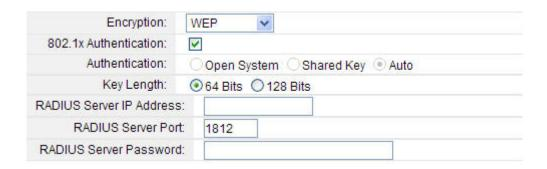
RADIUS Server IP Address: Enter the IP address of RADIUS server.
