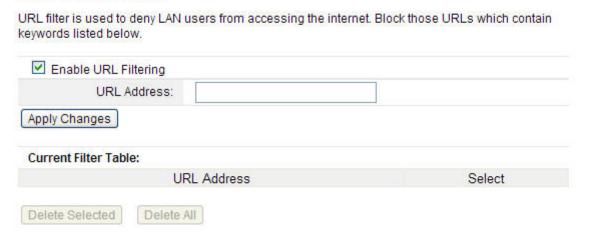
**Enable URL Filtering:** you can select this checkbox to enable URL filtering function. **URL Addresses:** type in the keywords contained in URLs that you don't allow LAN users to access.
