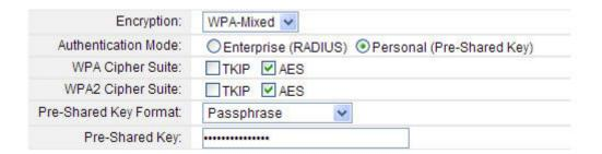
**Note:** Since WEP has been proved vulnerable, you may consider using WPA2 for the most secure connection. You should select the appropriate security mechanism according to your needs. No matter which security suite you select, they all will enhance the over-the-air data protection and/or privacy on your wireless network.
