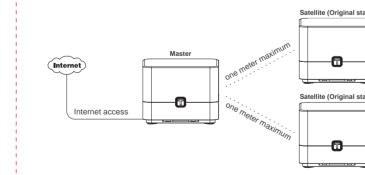
There are two methods of sync between one Master and two Satellites. One is achieved using the panel T button, the other via the Master's Web
