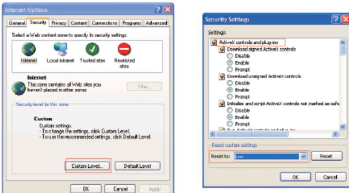
When using IE to preview network camera, you have to set the security level for ActiveX controls. Click [Tools] and choose [Internet Options] in the IE menu. Choose [Security] and click [Custom level...] to enter the “Security Settings” page, Enable ActiveX Controls and Plugins and choose low security level. For safety sake, reset to the “security level” to default values after the preview.
