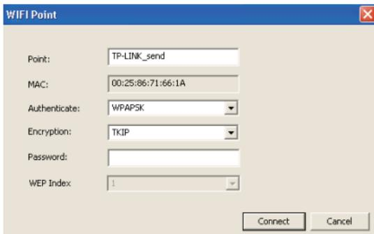
If entered this screen by double clicking, hotspot will be assigned automatically; if entered this screen by clicking [Add hotspot], user has to type in hotspot, corresponding encryption mode and password. Click [Connect], close the dialog box, and connected or not will be list on the research results list.
