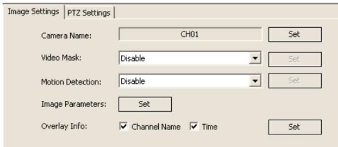
Please enter<Device parameters>-<Camera settings>-<Image> to set channel name. User can choose the suitable letter and size. In OSD, the channel name will be displayed on left upper corner when clicking [Channel name], and the channel time will be displayed on the righter corner of the screen when clicking [Time].
