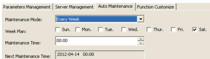
Enter [Device parameters/Device management...] screen, click pop-up [Maintenance] to set auto-maintenance mode to reboot the device for clearing redundant data.
