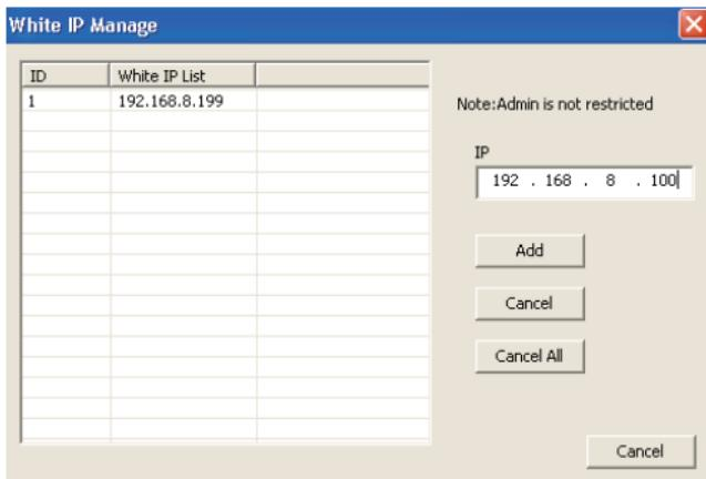
IP Filter: Set IP white list. While enable the IP filter, only the users on the PC with valid IP address in the white list can remotely log into the device.
