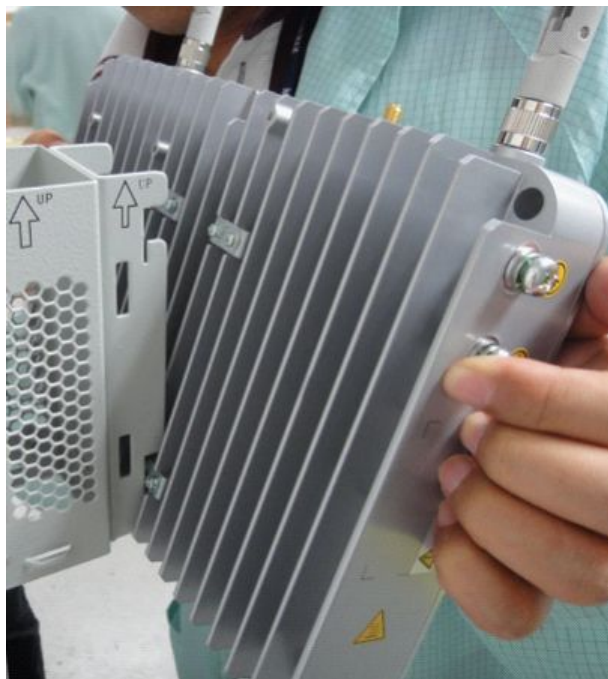
Figure 6-3 Hanging the ZXSDR BS8802 C100
