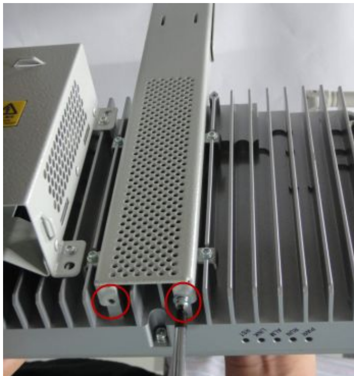
Figure 6-18 Fixing the ZXSDR BS8802 C100
