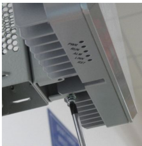
Figure 6-4 Fixing the ZXSDR BS8802 C100
