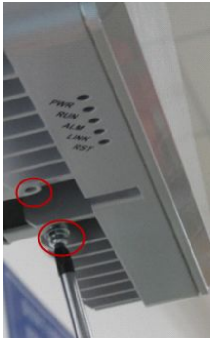
Figure 6-13 Fixing the ZXSDR BS8802 C100
