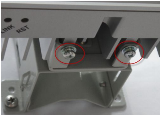
Figure 6-9 Fixing the ZXSDR BS8802 C100
