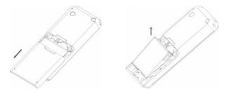
Install: Place the bottom of the battery into position, push down on the upper section of the battery until it clicks into place and then install the battery cover.
