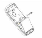
Install: Place the bottom of the battery into position, push down on the upper section of the battery until it clicks into place and then install the battery cover.
