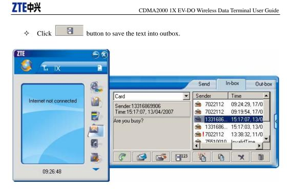
The received messages will be saved in the Data Terminal In-box. After the Data Terminal In-box is full, the system will automatically move the messages in the Data Terminal In-box to the PC In-box, and clean out the Data Terminal In-box.
