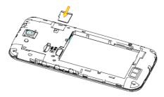
Insert the battery by aligning the gold contacts on the battery with the gold contacts in the battery compartment. Gently push down on the battery until it clicks into place.
