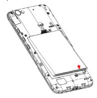
$5_{\times}$  Align the back cover with the back of the phone and press the cover back into place. Make sure all the tabs are secure and there are no gaps around the cover.
