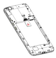
Hold your microSDHC card with the metal contacts facing down and slide it into the microSDHC card slot.
