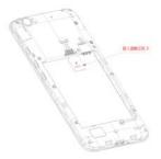
3. Insert the memory card into the card slot with the metal contacts facing down until it inserts to the right position.
