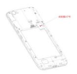
4. Insert the battery by aligning the gold contacts on the battery with the gold contacts in the battery compartment. Gently push down on the battery until it clicks into place.
