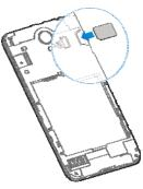
3. Hold your microSDXC card with the metal contacts facing down and slide it into the microSDXC card slot.
