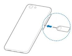
2. Pull out the card tray and place the micro-SIM card and an optional microSDXC card on the tray, as shown. Carefully slide the tray back into place.
