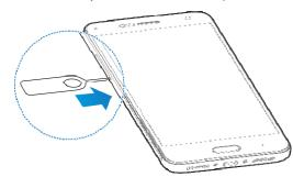
2. Place the nano-SIM/microSDXC card on the tray with the gold-colored contacts facing down. Then carefully slide the tray back into place.
