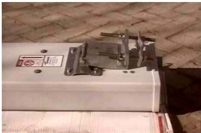
FIGURE 70 DIRECTIONAL-ANTENNA FIXATION CLIP
