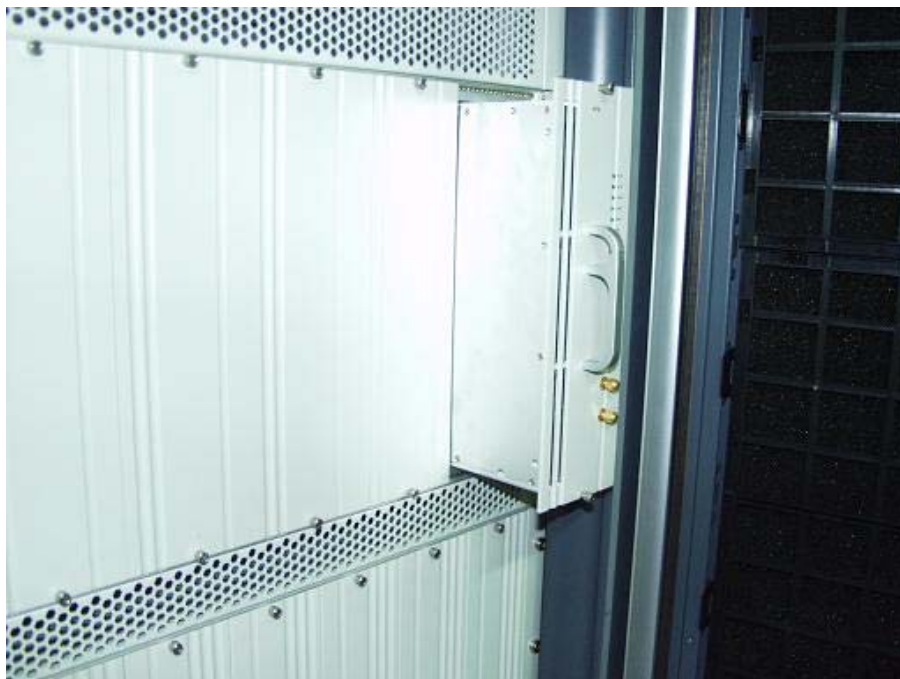
Fig. 12.3-3 Loosening the Screws and Unplugging the RFE
