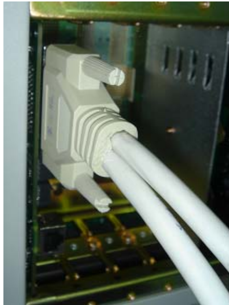
Fig. 8.1-1 D_SUB44-core Connector Connecting BDS
