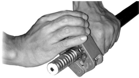
Fig. 10.4-7 Cutting the Feeder with a Cutter
