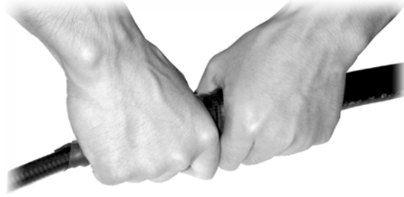
Fig. 10.6-3 Wrap the Waterproof Adhesive Tapes (3)
