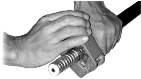
Fig. 10.4-7 Cutting the Feeder with a Cutter
