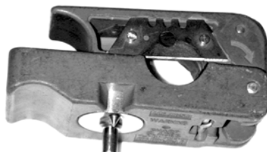
Fig. 10.4-6 Cutting Tool for the 7/8" Feeder Connector
