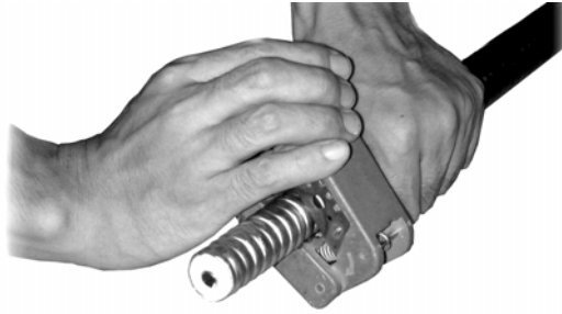
Fig. 10.4-7 Cutting the Feeder with a Cutter
