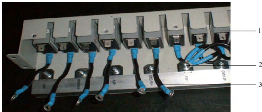
Figure G-3 Inside Cable to connect with PDM
