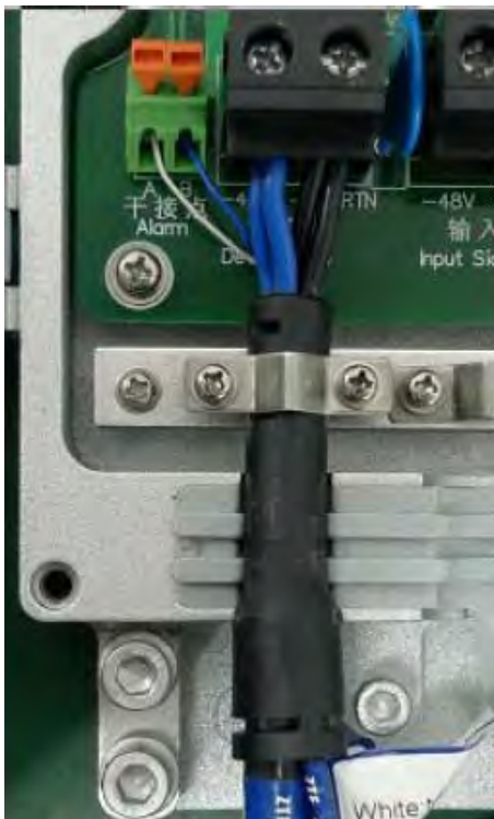
Figure 4-24 Connecting Output Power Cable and Dry Contact Cables
