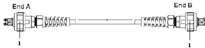
Figure 4-13 Fiber Connection between ZXSDR R8860s
