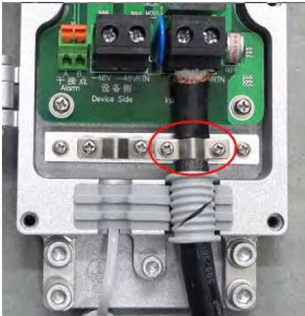
Figure 4-23 Connect Power Input Cable
