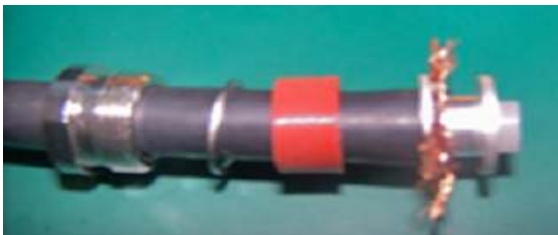
FIGURE 94 - INSERTING EXTERNAL CONDUCTOR FLANGE
