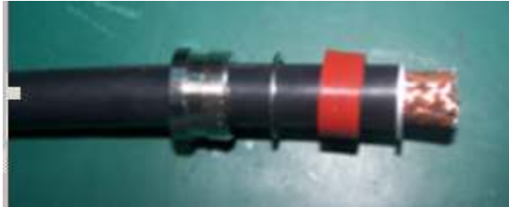
FIGURE 92 - EXTERNAL CONDUCTOR ASSEMBLY
