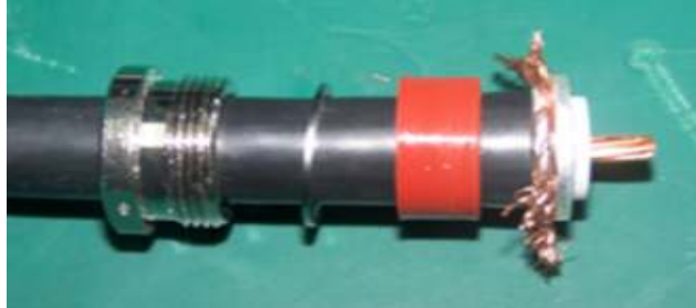
FIGURE 97 - INSERTING INSULATING PLATE
