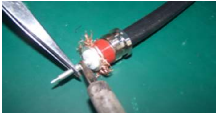
FIGURE 98 - WELDING INNER CONDUCTOR PIN
