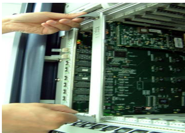
FIGURE 105 - BOARD PLUGGING (STEP 1)
