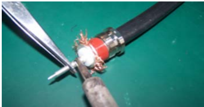
FIGURE 77 - WELDING INNER CONDUCTOR PIN
