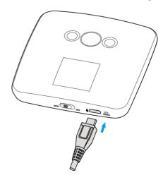
**NOTE**: The charge time varies depending upon the battery level. The device will stop charging if the temperature of the battery exceeds  $113 \, ^{\circ}F/45 \, ^{\circ}C$ .
