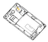
4. Insert the battery by aligning the gold contacts on the battery with the gold contacts in the battery compartment. Gently push down on the battery until it clicks into place.
