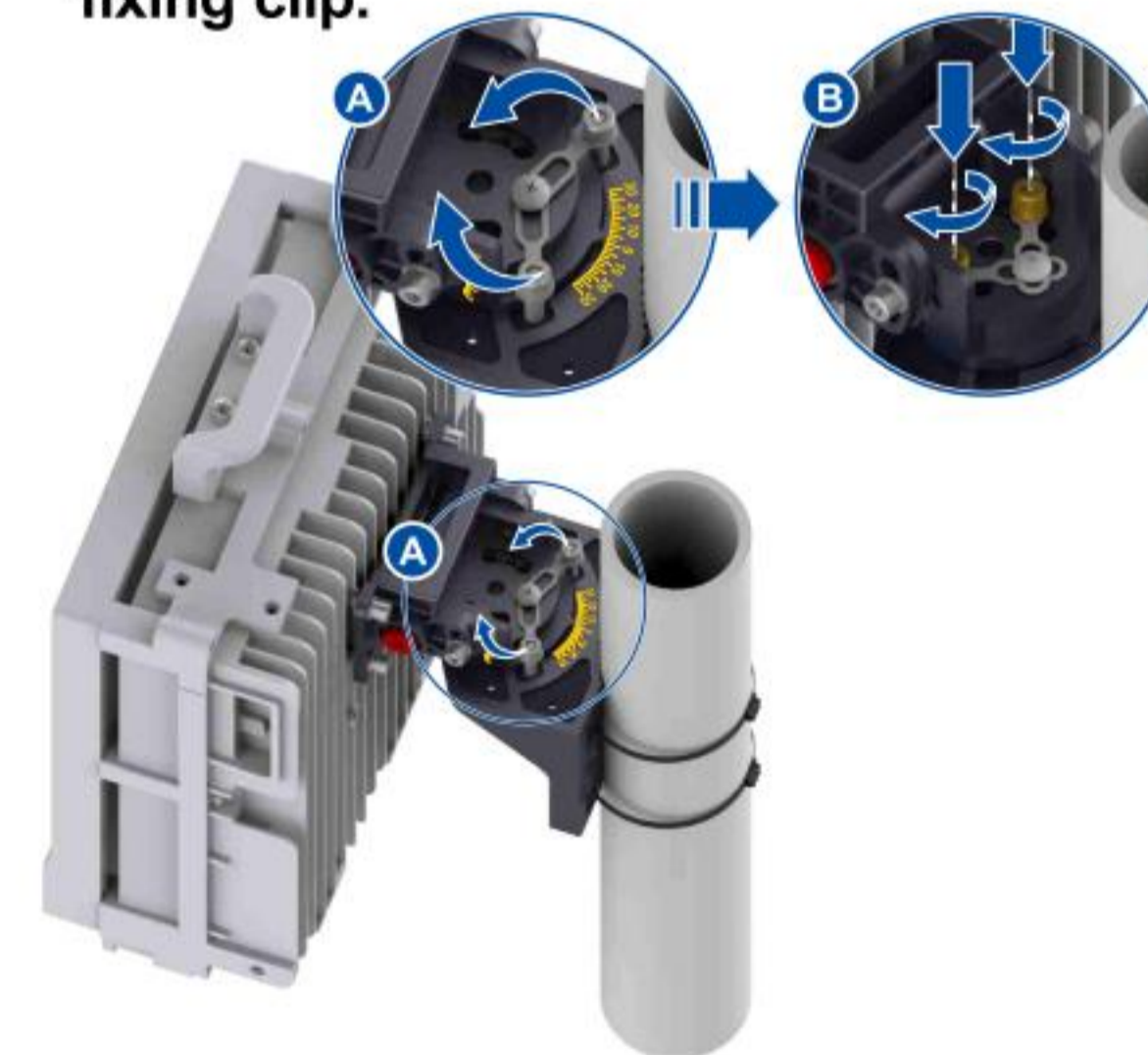
b Secure the two screws of the installation bracket on the fixing clip.
