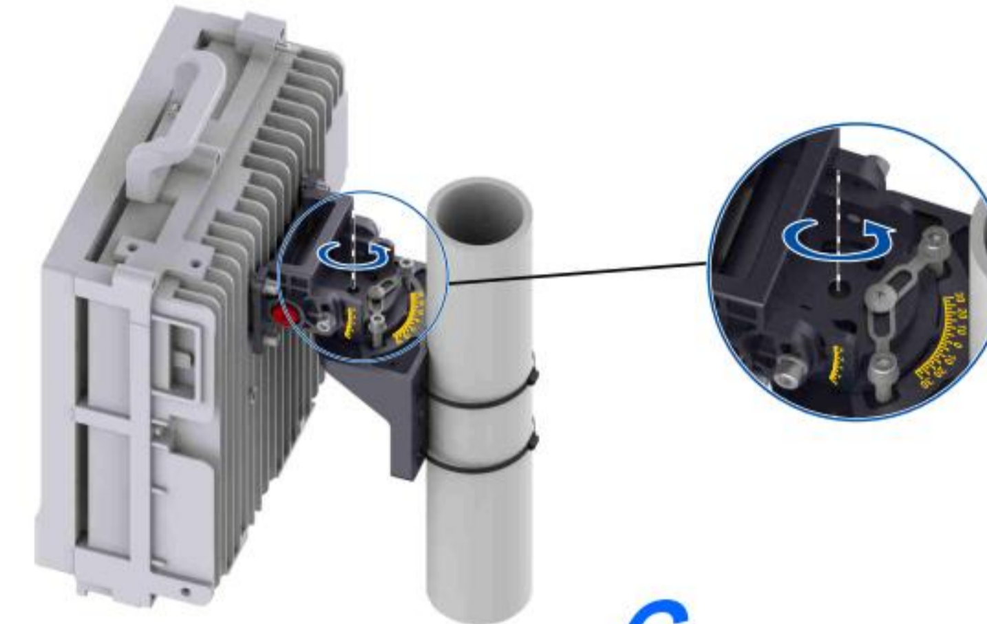
b Secure the two screws of the installation bracket on the fixing clip.
