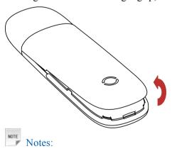
Do not open the front cover rudely so as to avoid the damage of the front cover.
