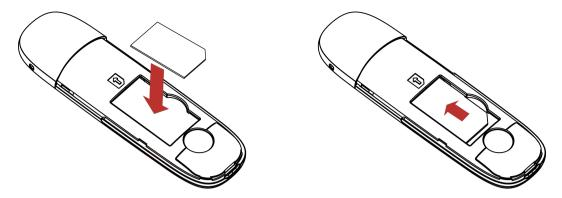
3. Put the front cover of the modem flatly upon the body of modem. Direct the front cover towards the locking catches on the sides of the modem and push the front cover of the modem to lock the front cover into its place.
