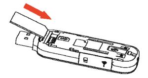
3. Put the front cover of the modem flatly upon the body of modem. Direct the front cover towards the locking catches on the sides of the modem, and then push the front cover of the modem to lock the front cover into its place.
