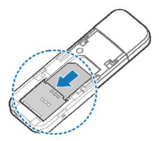
3. Insert the microSDHC card into the microSDHC card slot.
