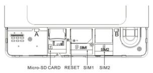
Install the cover in 45 degrees to point A and B as picture shows, press to fasten.
