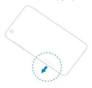
2. Hold the nano-SIM card/ microSD card with the cut corner oriented as shown and slide it into the card slot
