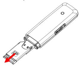
Then insert the SIM/USIM card into the socket, here make sure that metal contact area facing to the modem.
