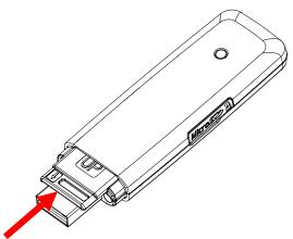
To Remove the SIM/USIM card from the USB modem
