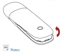
Do not open the front cover rudely so as to avoid the damage of the front cover.
