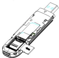
4. Put the front cover flatly upon the body of modem and push the front cover to lock the cover in its place.
