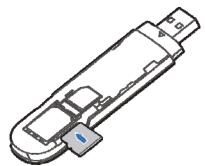
4. Put the front cover flatly upon the body of modem and push the front cover to lock the cover in its place.
