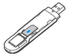
3. Insert the microSD card into the microSD card slot.
