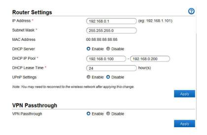
IP Address: The IP address for this device, as seen from the local network. This is set to a default value.
