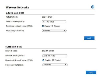
**Network Mode:** Indicates which mode is active for connecting via Wi-Fi. The default is 802.11b/g/n Mixed Mode for 2.4G network, and 802.11 a/n/ac Mixed Mode for 5G network.
