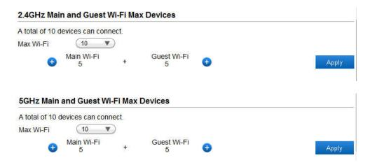
**Maximum Wi-Fi Devices:** Specify how many devices can simultaneously connect to the AT&T Home Base.
